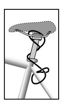
**STEP 1** Pass large loop through small loop around seat stay.
